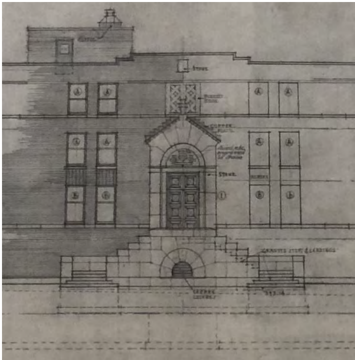
44. Ernest Cormier, 'St. Joseph's Street Elevations, March 1950, detail showing design and details of the central entrance bay and adjacent paired windows. (Ernest Cormier fonds, Canadian Centre for Architecture)
