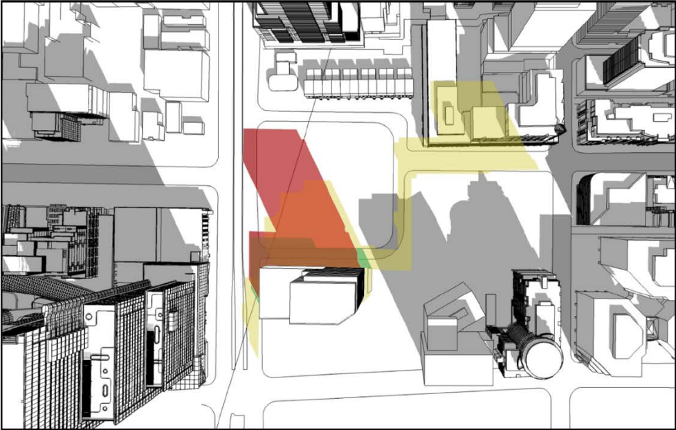
Shadow study of the original development proposal showing the extent of the shadow impact on Clarence Square Park
