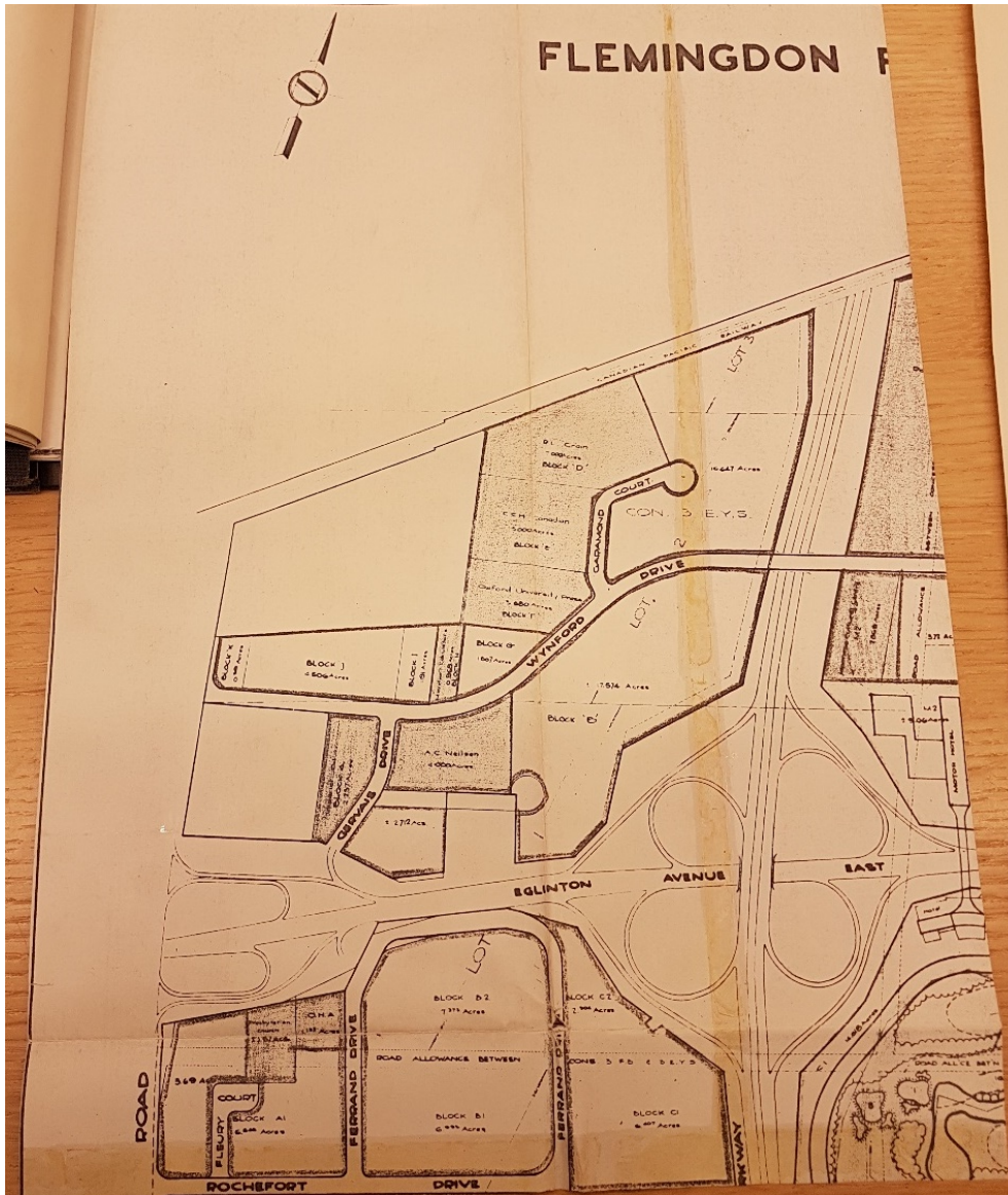
Figure 33: Excerpt from Flemingdon Park Master Plan showing proposed Industrial area, including Wynford Drive and proposed property owners, road layouts, and lot patterns. (Source: Knapp and Webb 1961).
